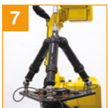
▲ RCST-90 robot diagnostic system, fitted in a working robot cell.
