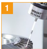
▲ OSP60 on-machine probe with SPRINT technology.
