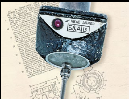
▲ The first touch-trigger probe and patent.
