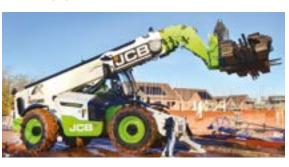
Vistry teamed up with JCB for one of the first onsite evaluations of its hydrogen-powered Loadall telescopic handler which was trialled on a project in Kenilworth.
