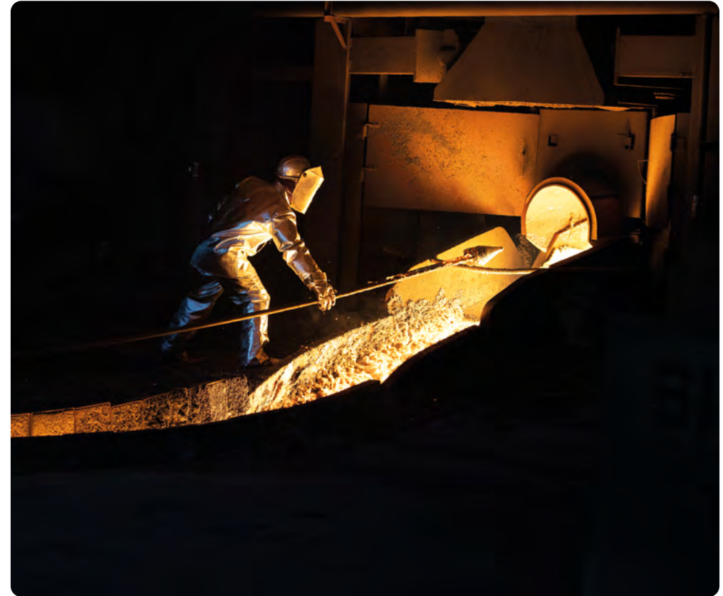
Molten metal is poured from a furnace at our Barro Alto operation, an important producer of ferronickel for the stainless steel industry.
