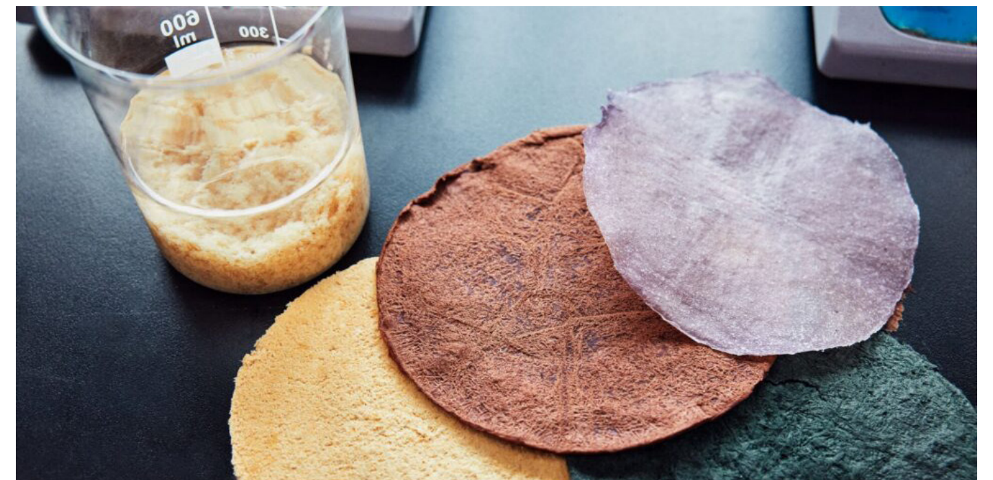
H&M Foundation. Recycled leather from leather scraps. Pictures from the HKRITA lab.
