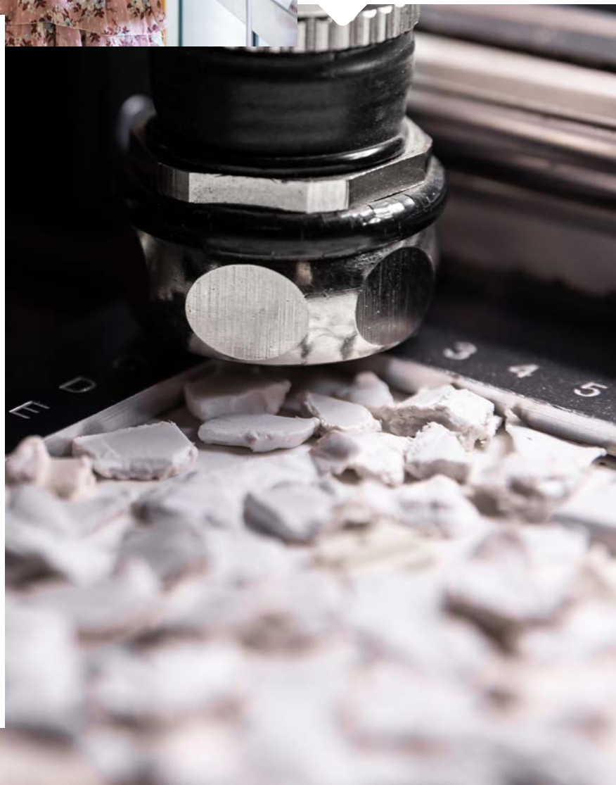
Quality testing polystyrene from recycled fridges at our Coolrec laboratory in Waalwijk, used in new fridges and Playmobil's Wiltopia range
