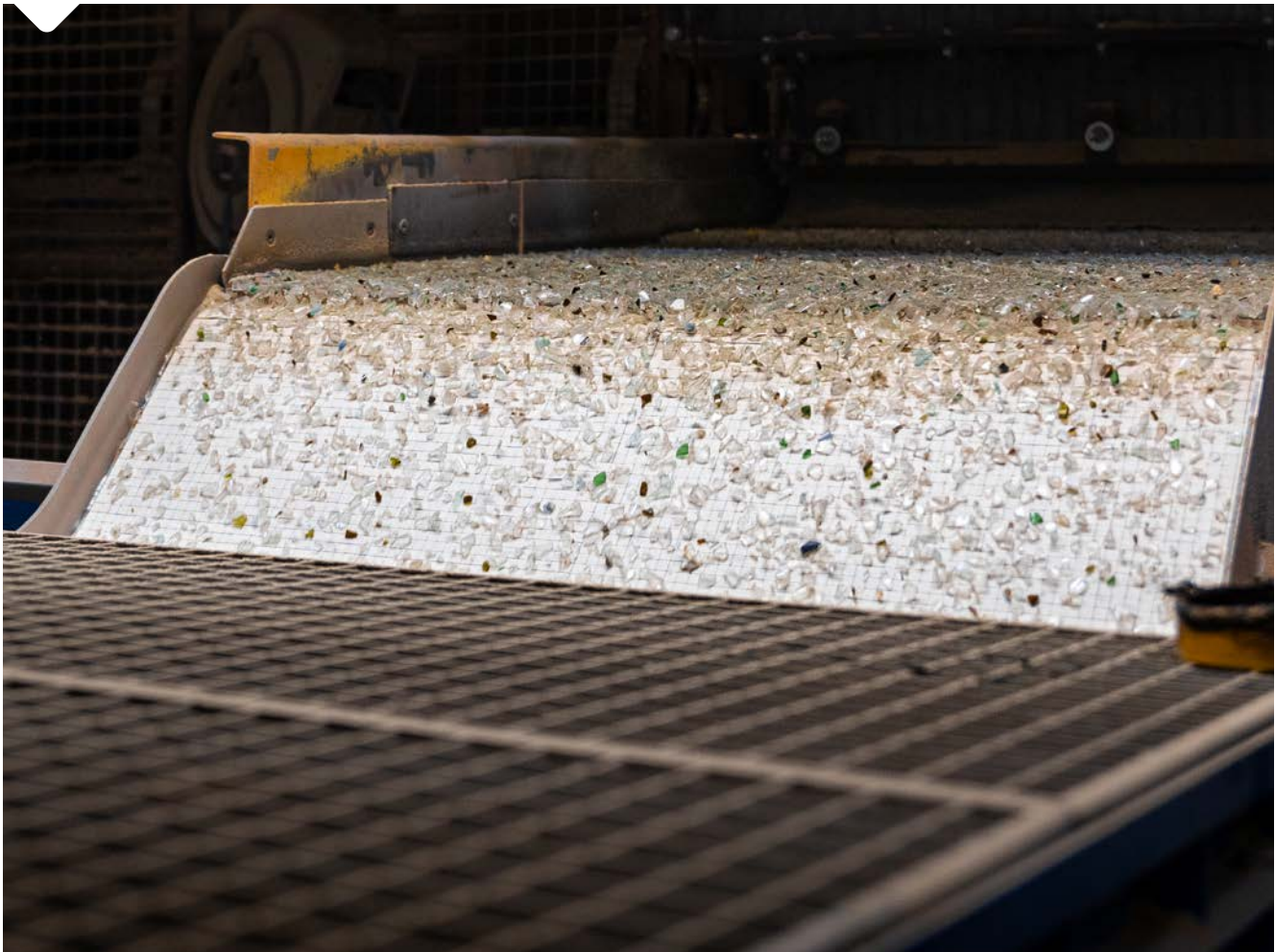
Optical sorting line, Maltha, Heijningen
