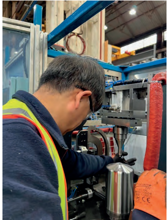
Trimming and polishing deep drawn stainless cans, Braime Pressings, UK.
