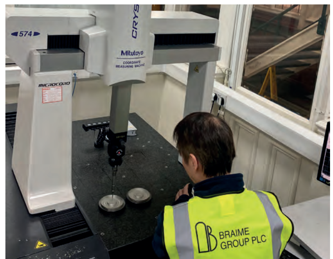
A coordinate-measuring machine (CMM) probing depth to the order of microns, Leeds, UK.
