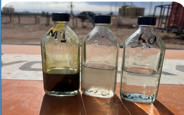
OIW Hexane Extraction Sample Left to Right: Inlet (37,868 ppm), MAC Outlet (184 ppm), REGEN Outlet (2 ppm)
