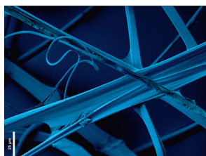
Image: The image depicts Silk Worm Cocoon and was prepared using the Q150T ES, applying a fine layer of Pt. For imaging, the Tescan Amber was used.
