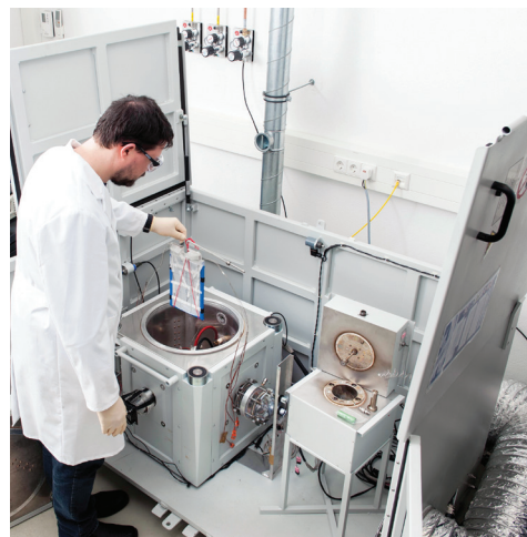
Image: Pouch cell battery being prepared for testing in THT EV+ ARC. Image courtesy of Dr Carlos Ziebert, Head of Battery Safety Centre, Karlsruhe Institute of Technology, Germany. © KIT/Almut Ochsman, Markus Breig.
