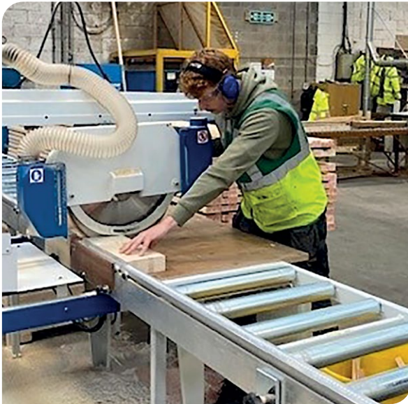
Radial arm saw in use at Dresser Mouldings.
