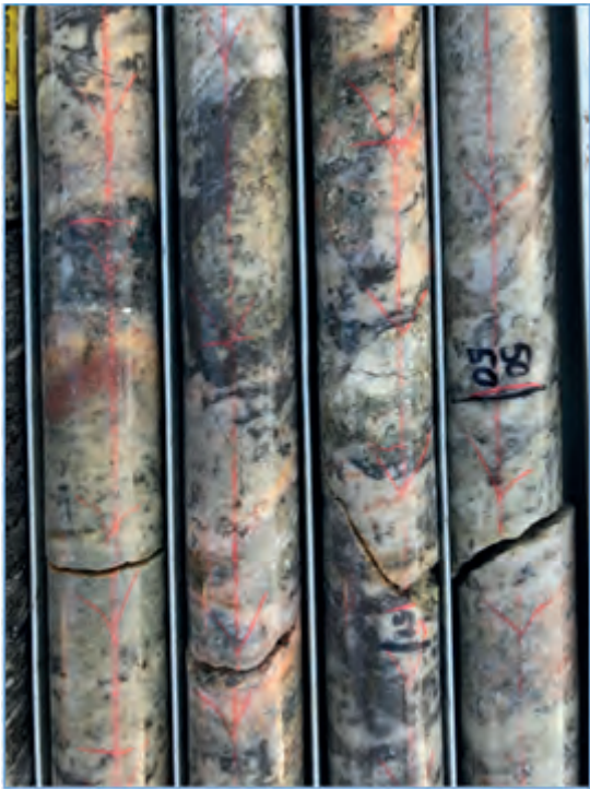
Photo 6: Kamativi pegmatite in drill core
