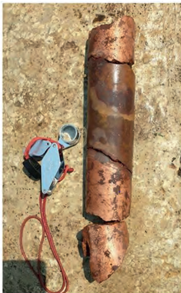
Photo 3: Drill core core with massive native copper from 103m depth in hole SHDD005
