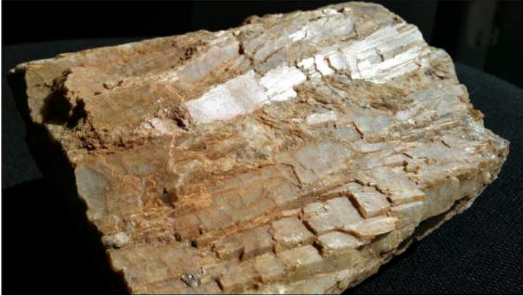
Figure 6-5: Wodgina Pegmatite Grey White Spodumene Crystals (Specimen Around 30 cm Long)
