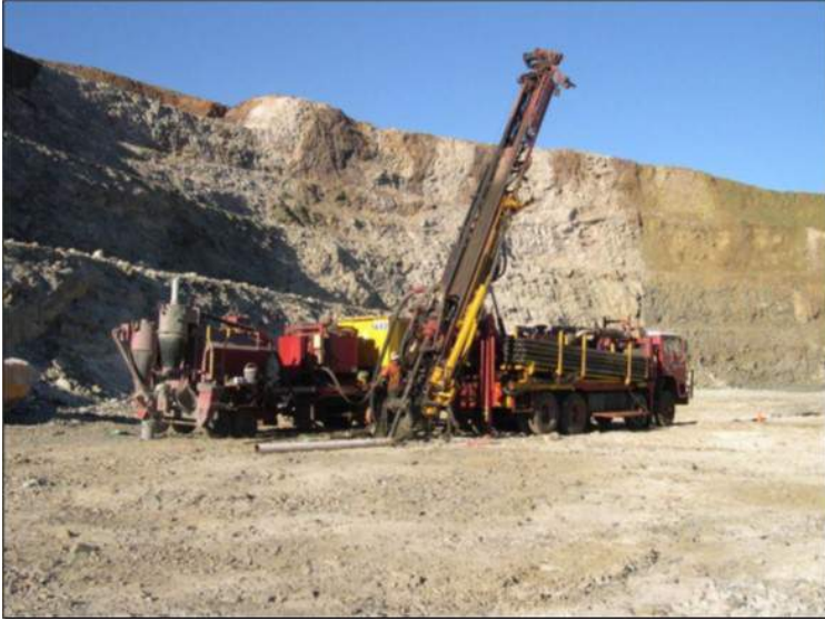
Figure 7-1: Magnet Drilling Hydro 150 Drilling RC in the Cassiterite Pit (During 2008)
